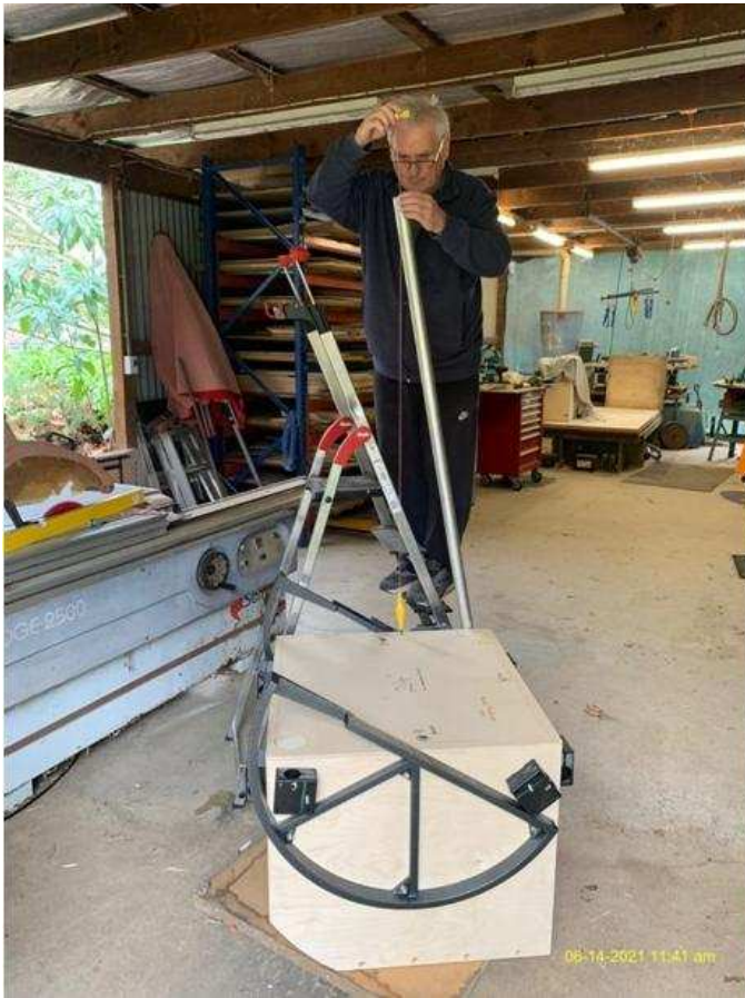
Measuring the angle of the truss poles.
