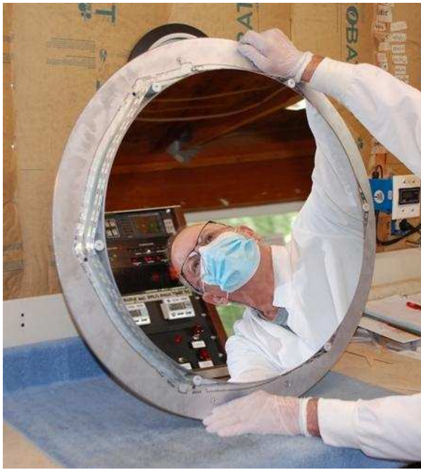
24" f/4 Quartz Mirror just out of the coating chamber.
