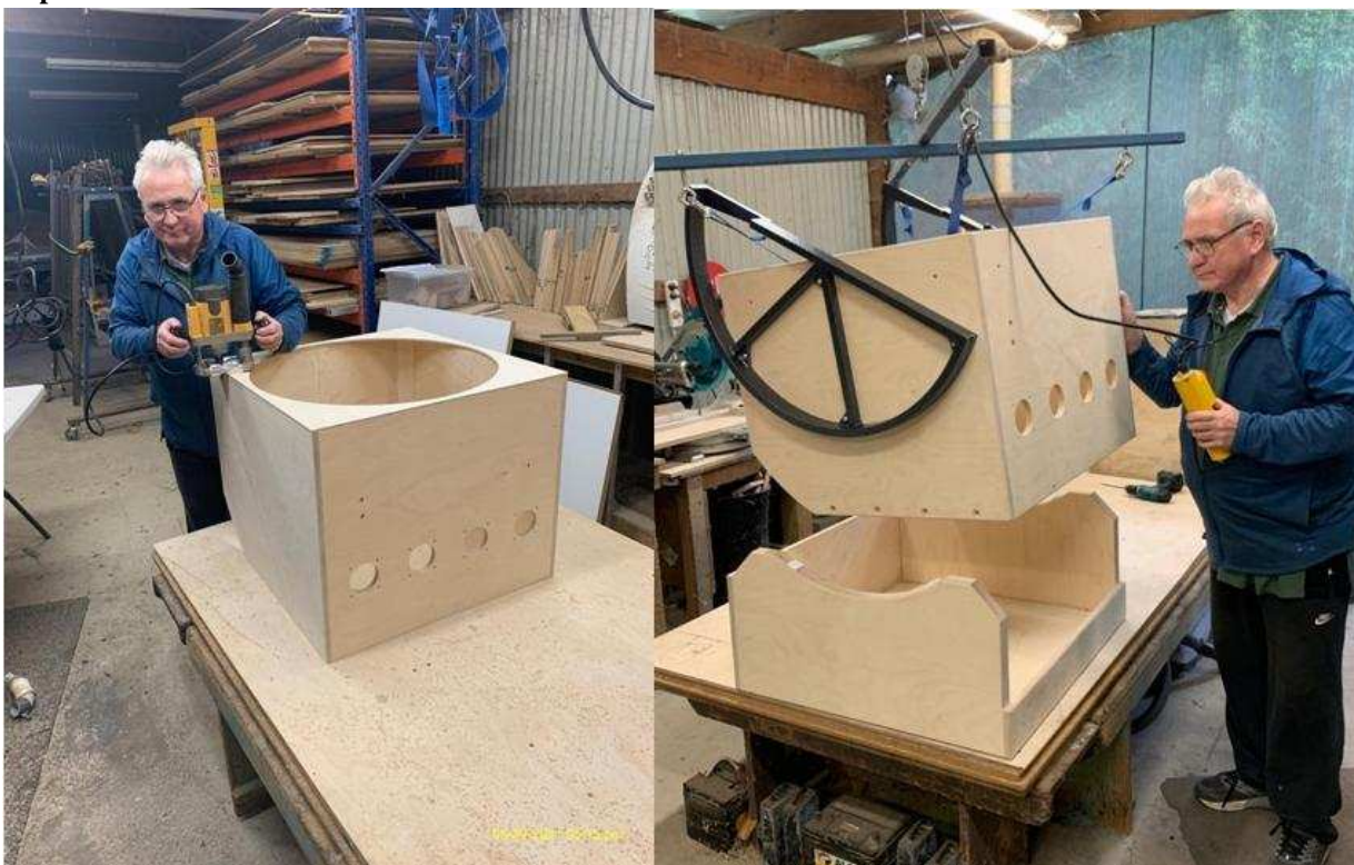
Pete starting the scope mirror box build and rocker box build. (I think a lot of my friends thought this might look like an expensive dummy)
